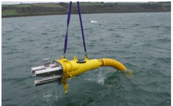
▲ Funded by ETI, MacArtney has developed and supplied an industry-first 11 kV wet mate connector. Providing a safe and reliable connection of renewable energy units and applications (such as wave energy converters, tidal energy converters and floating wind turbines to the power grid) the wet mate connector eliminates the need to bring cables to the surface. This shortens the time needed for connection, thereby making it possible to operate in waters with limited time windows.
