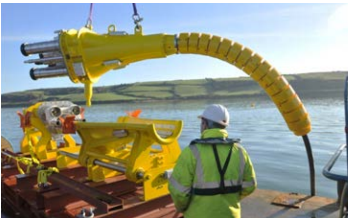
▲ Funded by ETI, MacArtney has developed and supplied an industry-first 11 kV wet mate connector. Providing a safe and reliable connection of renewable energy units and applications (such as wave energy converters, tidal energy converters and floating wind turbines to the power grid) the wet mate connector eliminates the need to bring cables to the surface. This shortens the time needed for connection, thereby making it possible to operate in waters with limited time windows.
