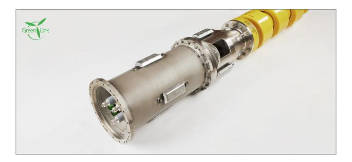
MacArtney GreenLink inline terminations have been designed to make offshore medium voltage termination jobs faster, easier and more efficient, hereby saving valuable ship time. These dry-mate systems are often used to connect dynamic cables from offshore renewable wind, tidal and wave energy converters to export cables. Moreover, they are widely used to interconnect subsea units.
